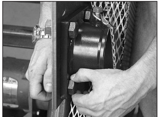
Remove the mounting spool from the non-tensioner side of the system. Line up the spool with the holes in the chute wall, then bolt it into place using four 3/4" grade 8 bolts and lock washers. You can also choose to stitch weld on the flat sides of the mounting spool.
