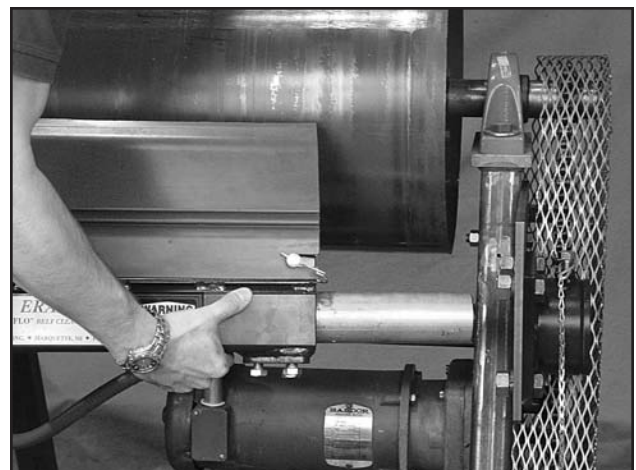
Lift the mainframe into position. Insert the stub end into the mounting spool on the non-tensioner side.
