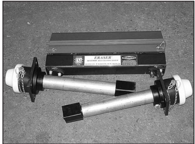
Remove both tension cartridges from the mainframe.
